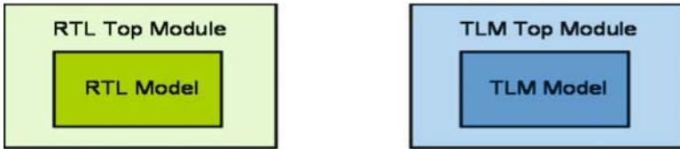
Figure 5-14. Separate Top Modules as Test Bench Platform
